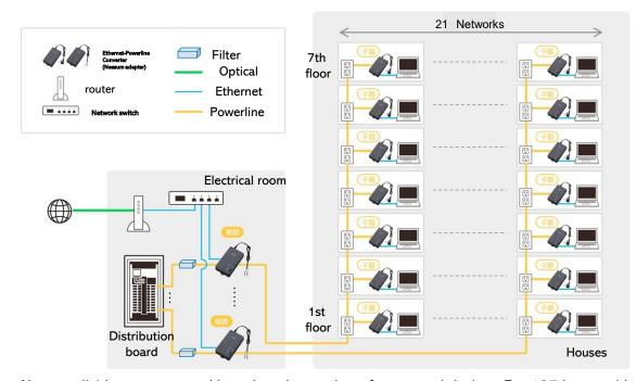
Nessum divides comm. speed based on the number of connected devices. For 137 houses, it's 146kbps per house. This is insufficient for remote classes, so filters are added to split each system, achieving 2.8Mbps per house. If high speed is not needed, filter costs can be reduced.
